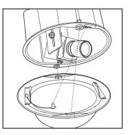
Figure 6. Installing the Lower Dome
